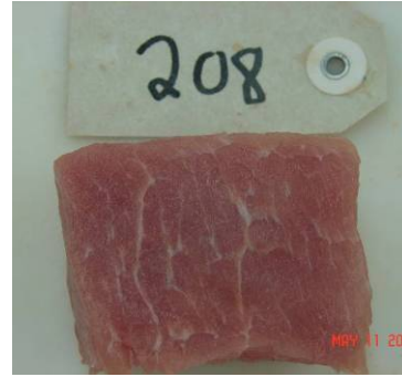
Figure 4 Tissue sample for chemical fat % determination of the scanned region of interest.
